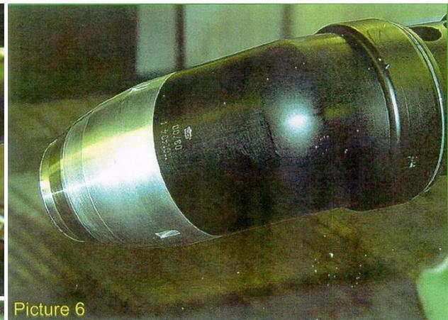
In Pictures 5, 6, & 7 we can see that, after a full hour of operation, there is still no condensation forming anywhere on the housing. Clearly, the condensation problem has been solved — permanently.
