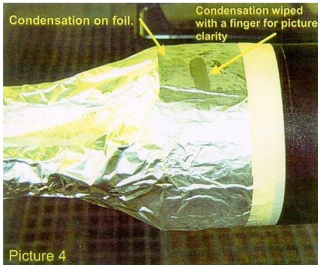
The formation of condensation can be predicted in any area where the surface temperature is below the 73.4°F dew point. These points were measured as shown here:
