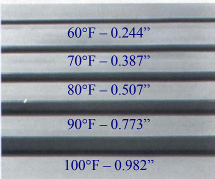
Figure 4: Extruded Adhesive Test
